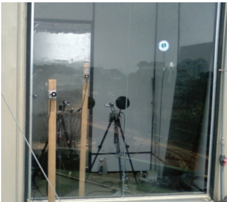
Figure 8: The view of the tested west facade showing the pyranometers that measure the internal/external vertical solar radiation of the CG façade.
