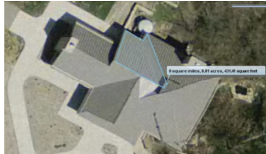
FIGURE 62: Over 430 square feet of roof runoff is directed to the rain barrel. Photo courtesy Hancock County Auditor, < http://hancock.iviewauditor.com >.
