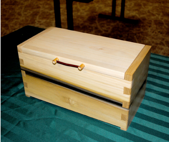
FIGURE 26: Poplar box with bamboo handle by student, Chun Yin Au. The box is a required project for all beginning woodworking students, and made from locally sourced poplar using only hand tools.
