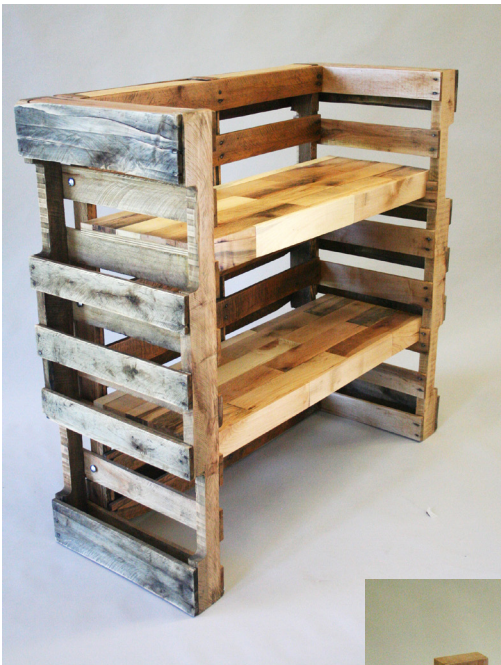
FIGURE 27: Pallet wood storage unit by student, Jack Dugan. Using pallets from campus dumpsters, he cleaned, sanded and modified them to fit the design of the piece.
