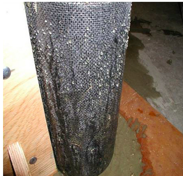
FIGURE 8: Bled clear water from the walls of a fabric formed concrete cylinder after casting.
