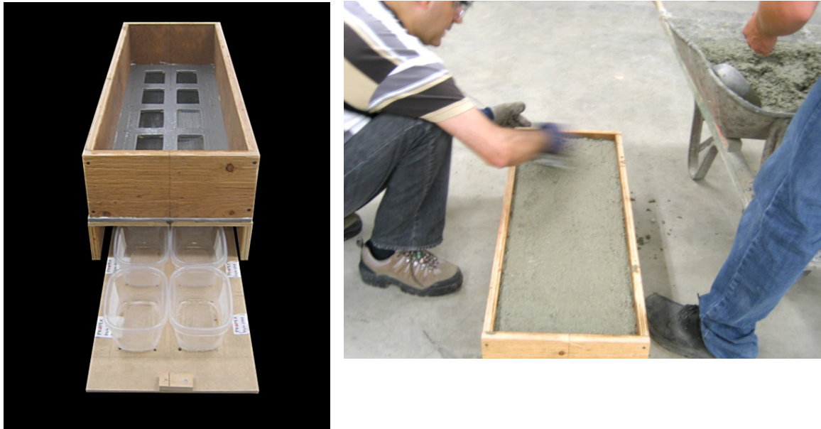
FIGURE 1: Test setup for box test.
