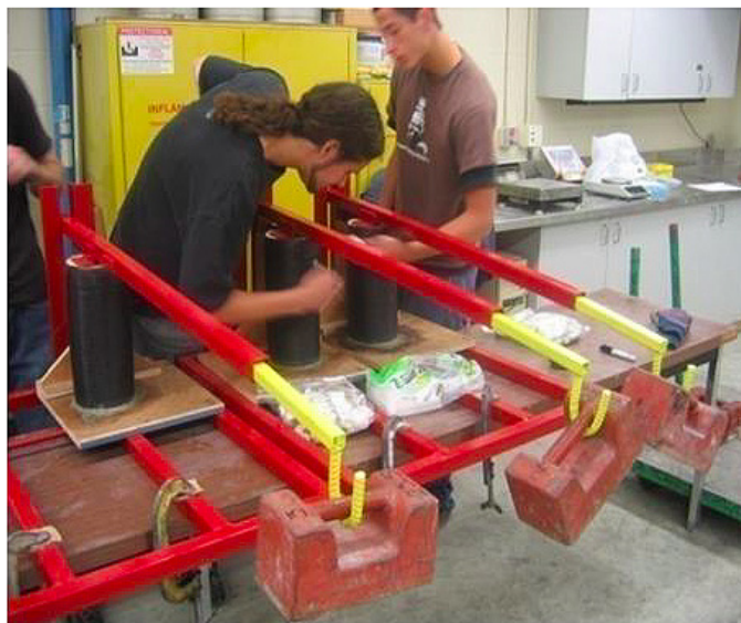
b) Collection of bleeding water during the bleeding test.
