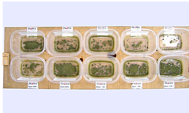
FIGURE 2: Collected cement and water bled through the fabrics.
