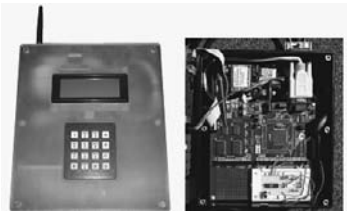
FIGURE 3. The outside (left) and inside (right) of the AWARE@home signal processing and communication board in its prototype form. Commercial implementation could reduce its volume by a factor greater than 10.
