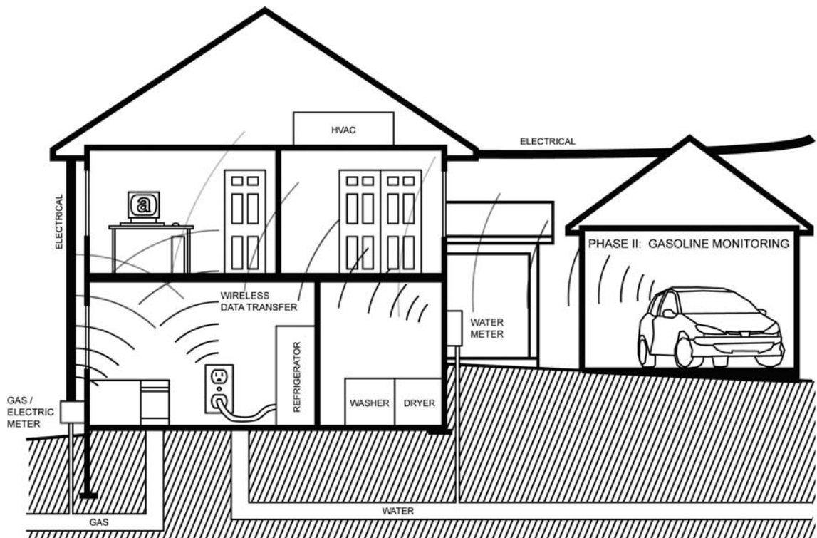
FIGURE 1. Conceptual illustration of the AWARE@home system. Digital flowmeters, microprocessors, and wireless transmitters are incorporated within existing metering technologies (gas, electric, water) so that consumption data and alarms can be sent to an in-home personal computer. Also shown is a wireless meter that can communicate the electricity consumption of individual appliances “plugged in to the wall” to the AWARE@home system.
