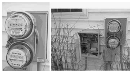
FIGURE 11. (Left) Meters running side-by-side to assure that AWARE@home system does not cause meter to “run slow”. (Right) Prototype manifestation of AWARE@home system using off-the-shelf components as installed at the test home.
