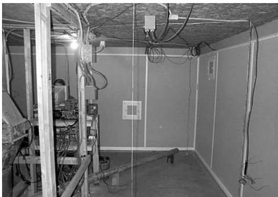
FIGURE 2. Test configuration for evaluating an insulation system using coarse-weave polyolefin covered semi-rigid fiberglass insulation.
