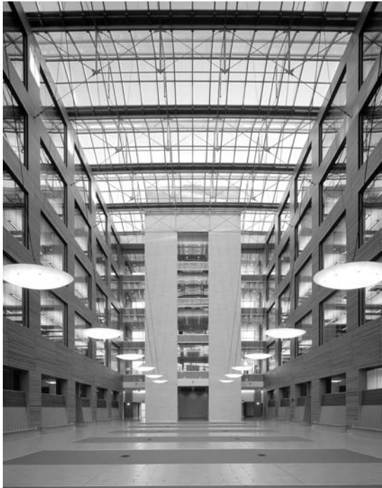
FIGURE 17. The atria reduced the area of envelope exposed to the elements and enhanced daylight penetration into the labs. (Photo: Elizabeth Gyde, DSAI.)
