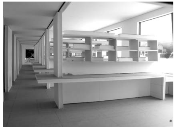
FIGURE 19. Daylight testing for Labs using scale model. (Photo: Lighting Design Lab, Seattle.)
