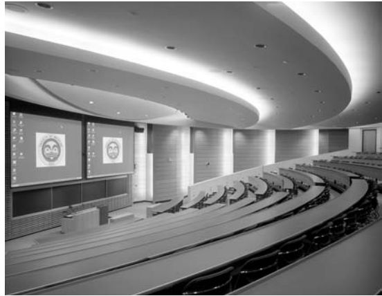
FIGURE 21. Air in the 350-seat lecture theatre is delivered under the stepped rows of seating at very low velocity. (Photo: Howard Waisman.)
