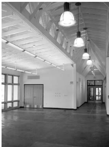
Commons Area with stained concrete floors and exposed trusswork.
