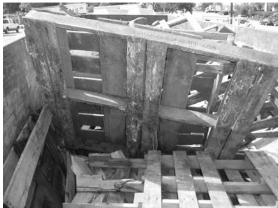
FIGURE 3. Photo of a wood recycling dumpster in Columbia, SC with significant bridging.
