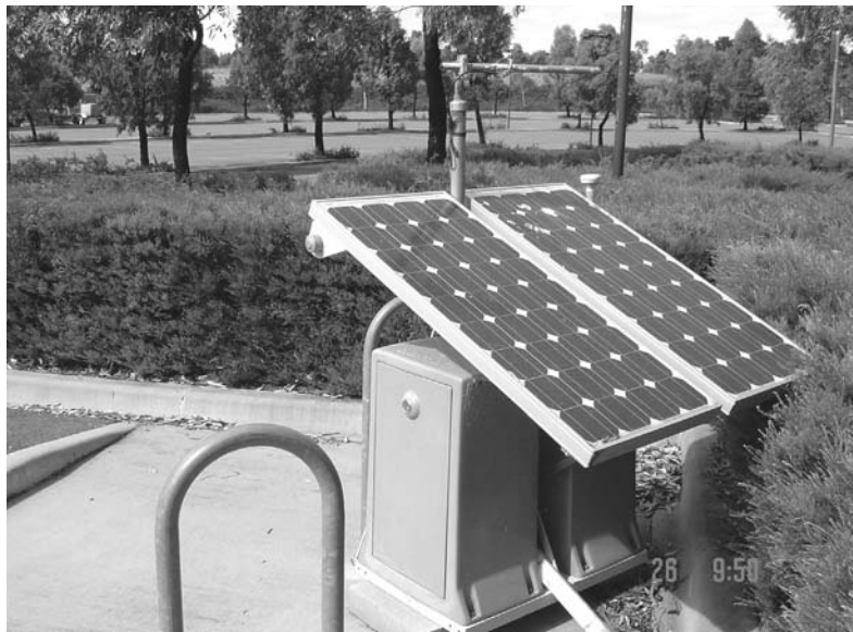
FIGURE 4. Locating an antenna directly above the photovoltaic modules that power this earthquake monitor has provided an ideal perch for birds to generate partial shading on the glass front cover below.
