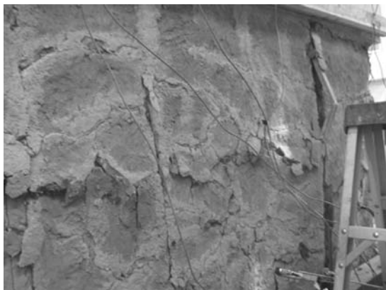
FIGURE 11. Failure cracking of wall.
