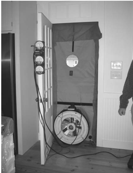
FIGURE 7. Testing the house's air leakage using the blower door test.
